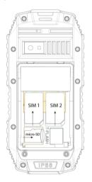
slot contacts. The phone uses mini-SIM cards. Insert a compatible memory card in accordance with the instructions in the picture. This device supports micro-SD memory cards up to
