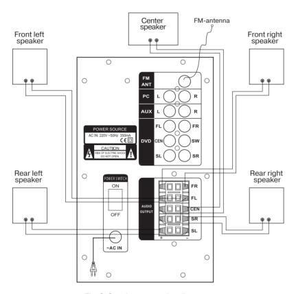
Fig. 6. Speaker connection diagram
