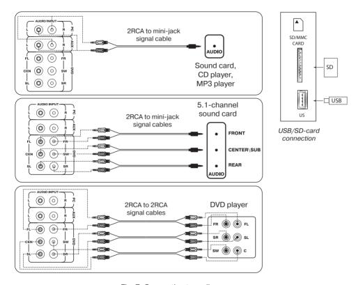
Fig. 7. Connection to audio sources
