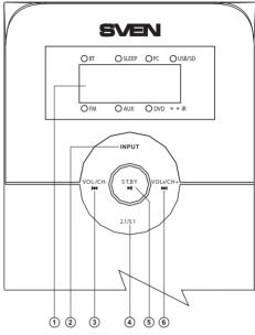
Fig. 1. Subwoofer control panel
